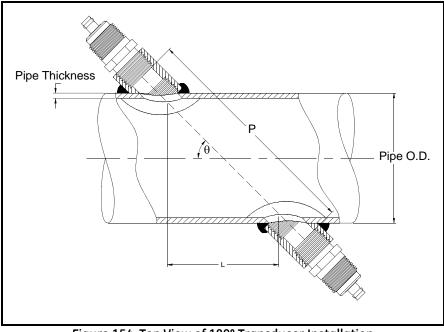
Figure 154: Top View of 180° Transducer Installation
